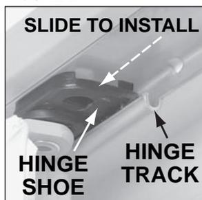
2. Place hole in the top hinge arm under the top track pin. Push up to seat arm on pin. Place a standard screwdriver into the slot on the retaining clip and slide toward track pin until it snaps into place.
