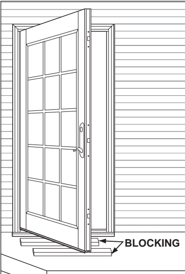
FIGURE 2 Outswing Hinge Viewed From Interior
