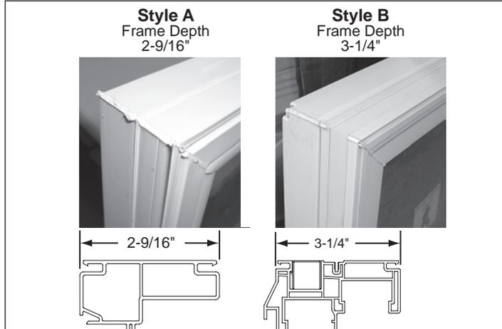
These instructions apply to the window styles shown above (FIGURE 1). Style A comes only as a single or double hung. Style B can be purchased as a single hung, double hung, awning, casement, or single, double, or triple slider.
