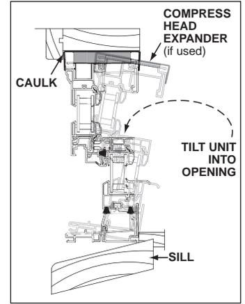
**IMPORTANT:** For proper support, mullied units must be shimmed under each mull joint as well as at the end side jambs.
